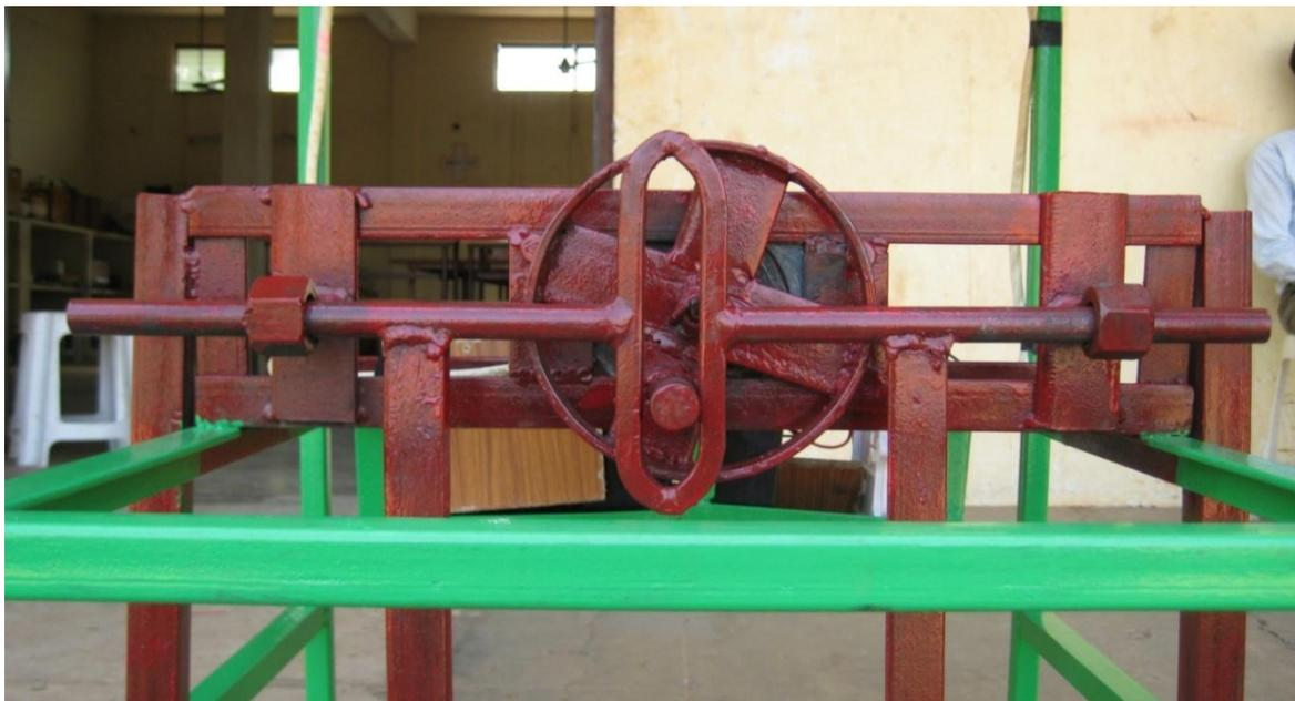
Figure 7 scotch yoke mechanism
