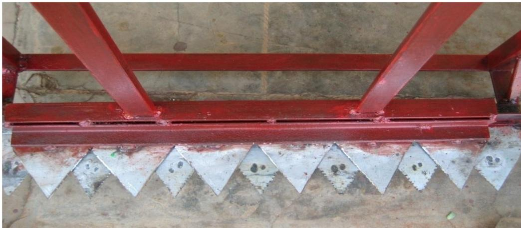
Figure 9 showing sliding and moving blade
