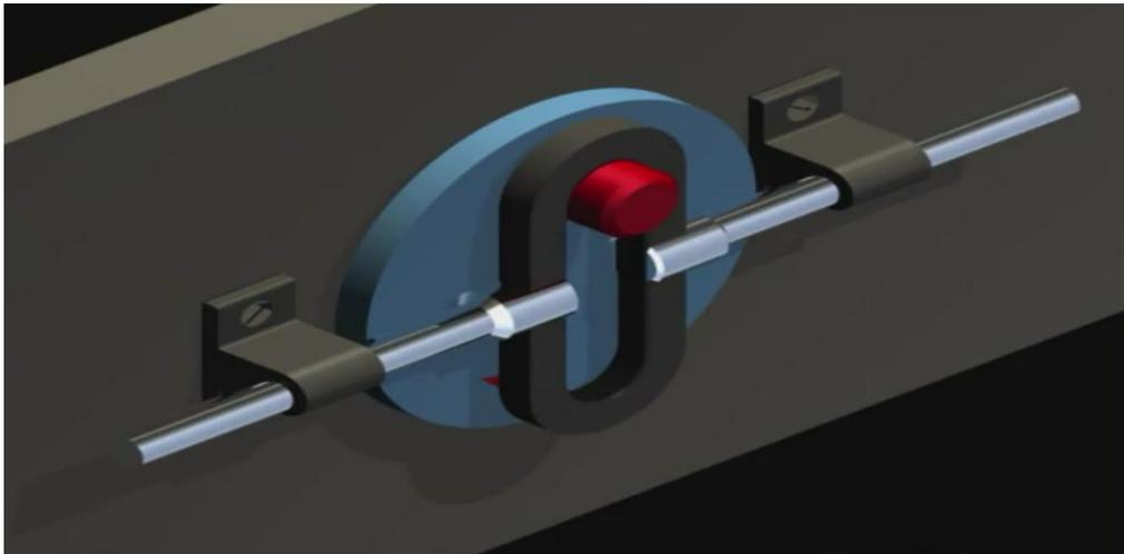
Figure 6 animation view of scotch yoke mechanism
