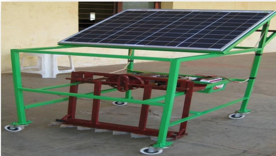
Figure 1 solar grass cutter with linear blades
