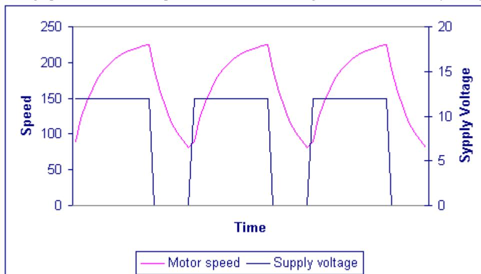
We can see that the average speed is around 150, although it varies quite a bit. If the supply voltage is switched fast enough, it won't have time to change speed much, and the speed will be quite steady. This is the principle of switch mode speed control. Thus the speed is set by PWM – Pulse Width Modulation.
