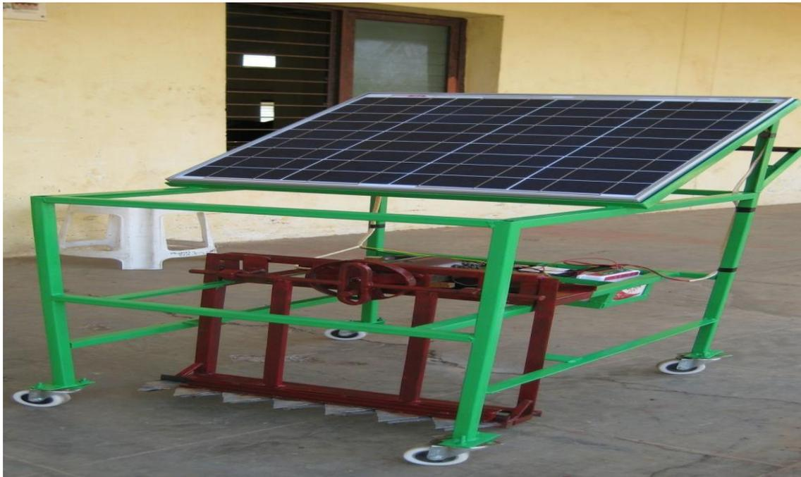
Figure 10 orthographic view of solar powered grass cutter
