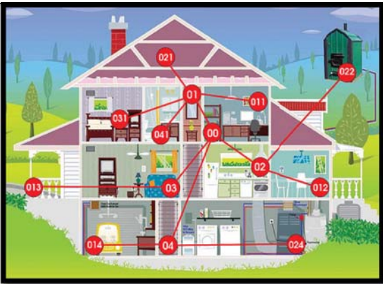
Figure 11. Diagram from ManiacBug showing the addressing of the RF24Network nodes
