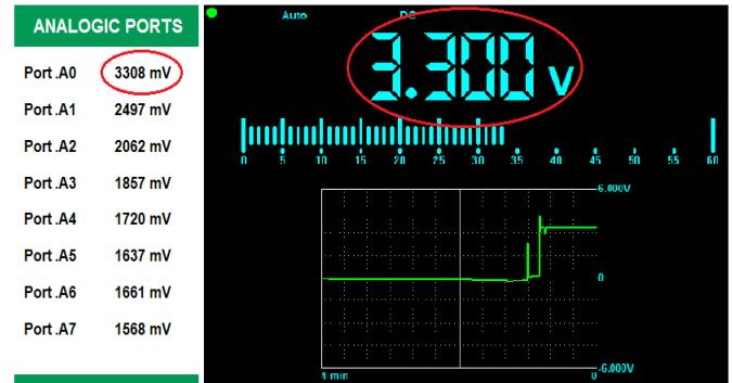
Fig.17 Display the voltage of to ADC, input port, A0
