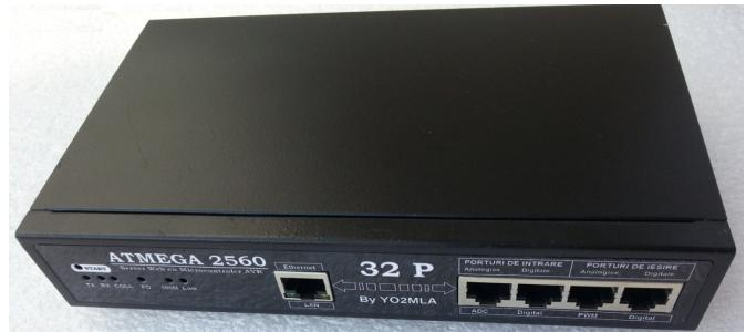
Fig. 15. The front panel of the prototype built Web server
