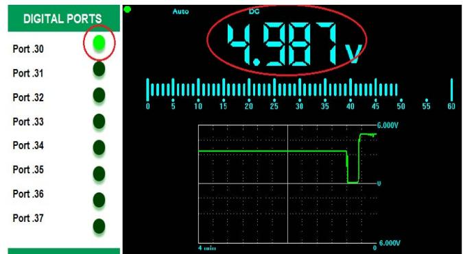
Fig.19 Displaying the logical 1, digital input port, P30
