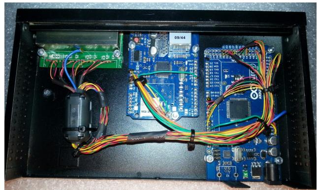
Fig. 14. The interconnection of hardware components of the Web server
