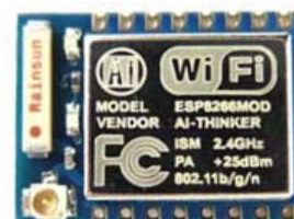
Fig 5. ESP8266-07 wifi serial transceiver module.
