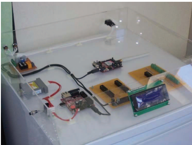
Fig. 2. The GSM enabled embedded electronic system mounted onto the refrigerator.
