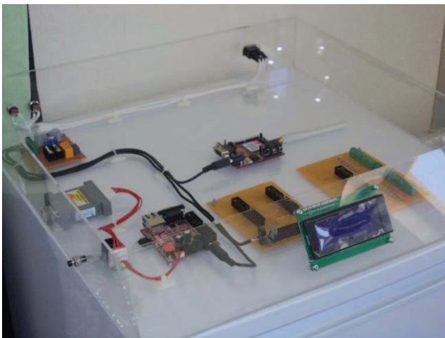
Fig. 2. The GSM enabled embedded electronic system mounted onto the refrigerator.
