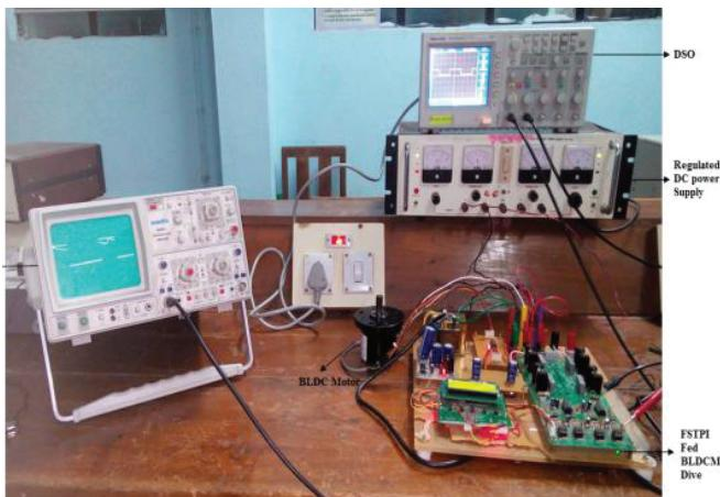
Fig 21: Complete photograph of hardware set up
