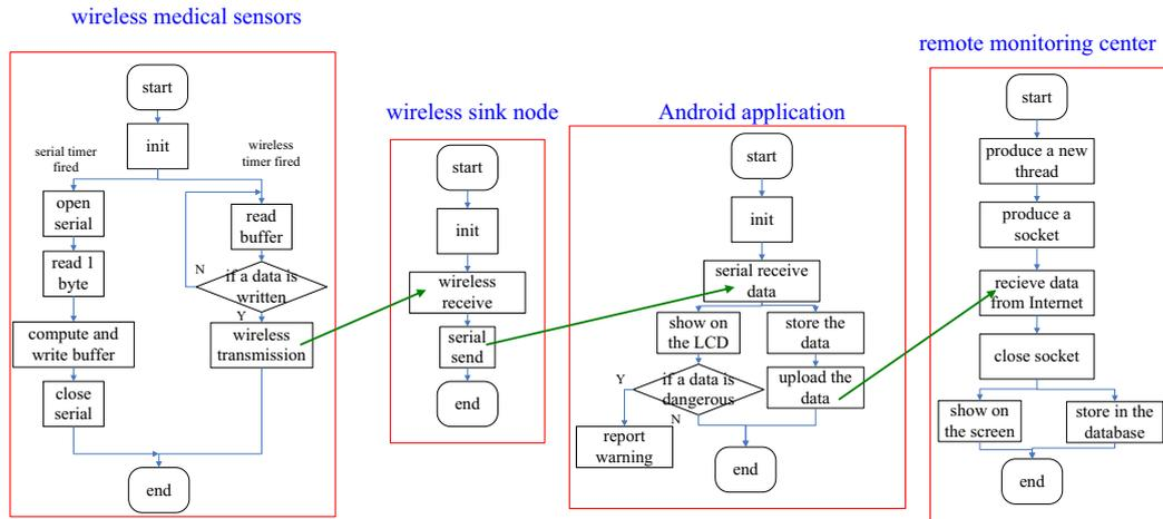
Fig. 3. The program flow diagram of the proposed system. Green lines indicate the flow direction of the data.
