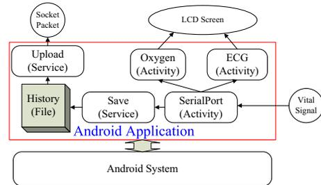
Fig. 7. The signal stream among the components of the Android application
