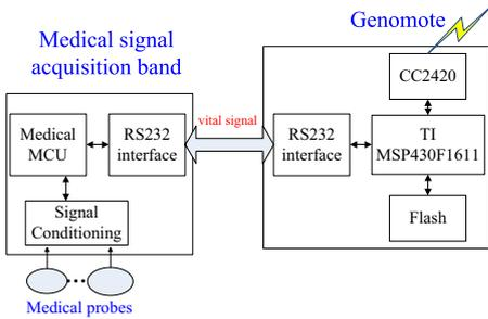
Fig. 4. The block diagram of the wireless medical sensors
