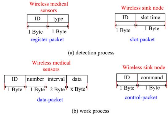
Fig. 6. The packet protocols of the sensor network tier.(a) in the detection process, (b) in the work process.
