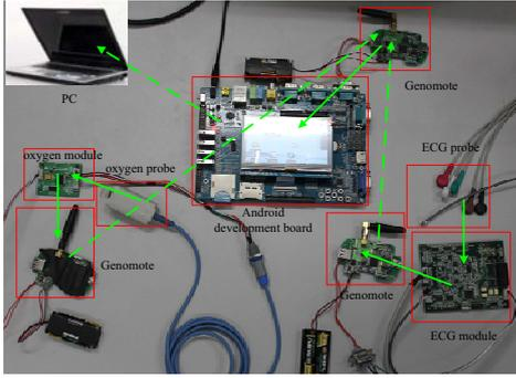
Fig. 2. The picture of the laboratory testing. Green lines indicate the flow direction of the data, thereamong solid lines represent wired transmission, dotted lines represent wireless transmission.
