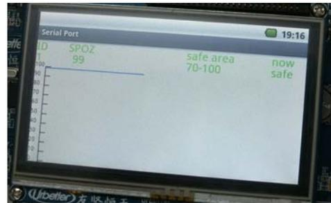
Fig. 8. The blood oxygen curve on the Android development board
