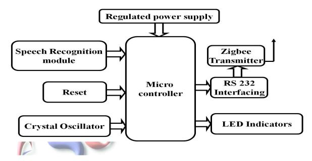
Zigbee based wireless Voice to Text translator in Airlines/Hospital assistant system for blind/Illiterates.
