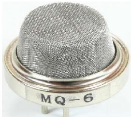
Fig. 4. The LPG Gas leakage sensor MQ6
