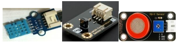
Fig. 5. DHT11 humidity sensor, LM35 temperature sensor, and MQ7 Carbon Monoxide gas sensor
