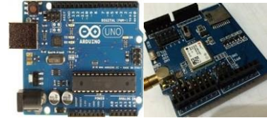
Fig. 6. Arduino Uno and GPS Shield
