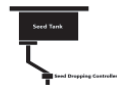
Figure 11. Seed Dropping Mechanism
