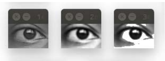
(a) Color image, (b) BGR to Gray conversion image, (c) Thresholding on image. Fig. 6.2
