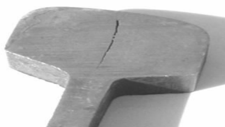
FIGURE 4. LONGITUDINAL VERTICAL CRACK
