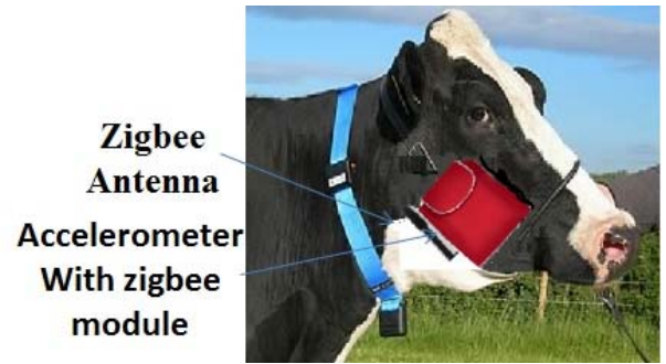
Fig. 14. Experimental setup of rumination sensor module.
