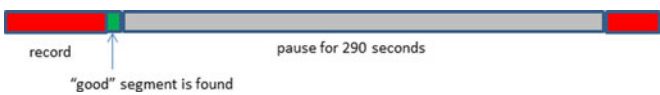
Fig. 5. Strategy B. As soon as a “good” segment of data is recorded, we pause for 290 s. At the end of the 290 s, we start recording again.
