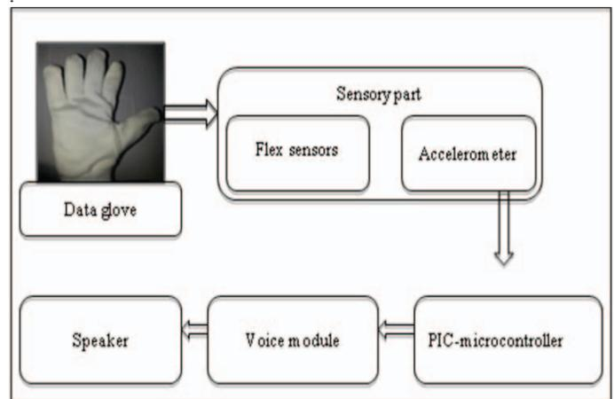
Fig. 1. Block Diagram of the ISL hand gesture recognition system
