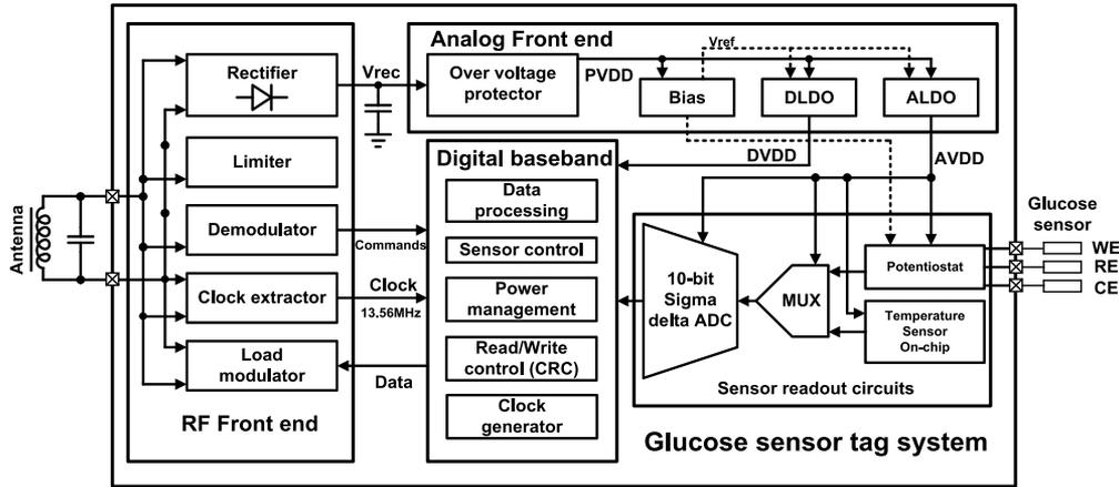
Fig. 2. Block diagram of the wireless sensor tag architecture.
