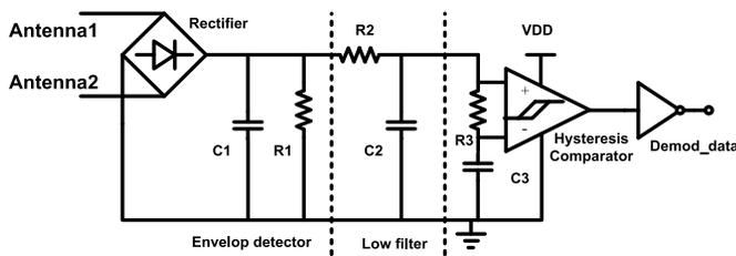
Fig. 5. Block diagram of the demodulation circuit.
