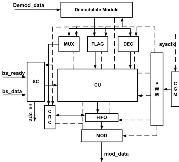
Fig. 14. Block diagram of the digital baseband.
