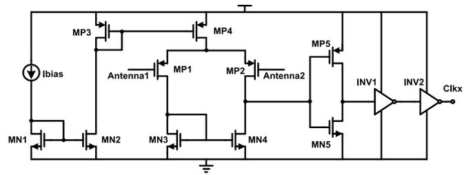
Fig. 6. Schematic diagram of the clock extractor.
