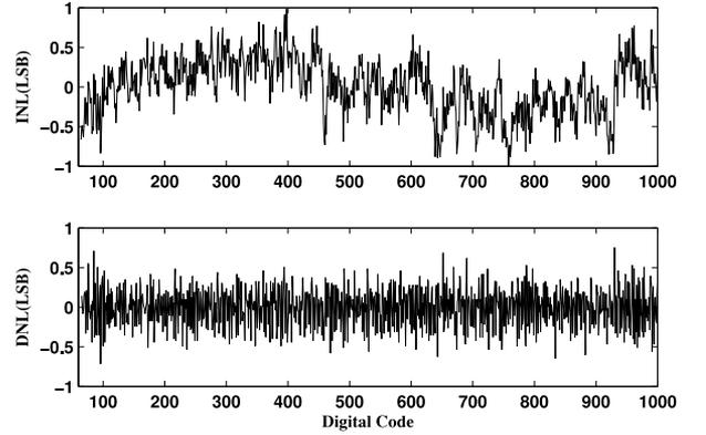
Fig. 13. Measured the 10-bit sigma-delta ADC static characteristic.
