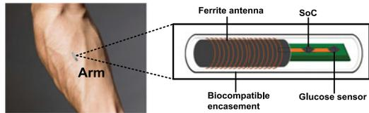
Fig. 1. Wireless powered implantable sensor tag for continuous glucose monitoring. The microsystem includes a ferrite antenna, a system-on-chip (SoC), and an electrochemical glucose sensor.
