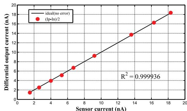
Fig. 9. Measured potentiostat differential output current versus sensor current.
