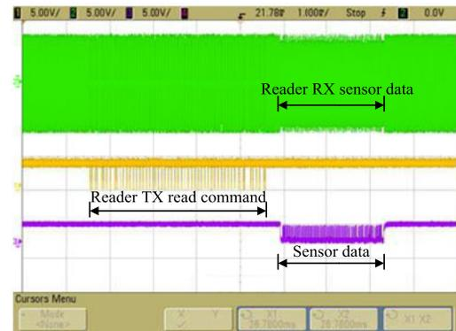
Fig. 17. Measured waveforms of the demodulated command, backscattered sensor data by load modulation, and voltage of reader antenna.
