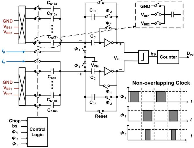
Fig. 11. Schematic diagram of the sigma delta ADC.
