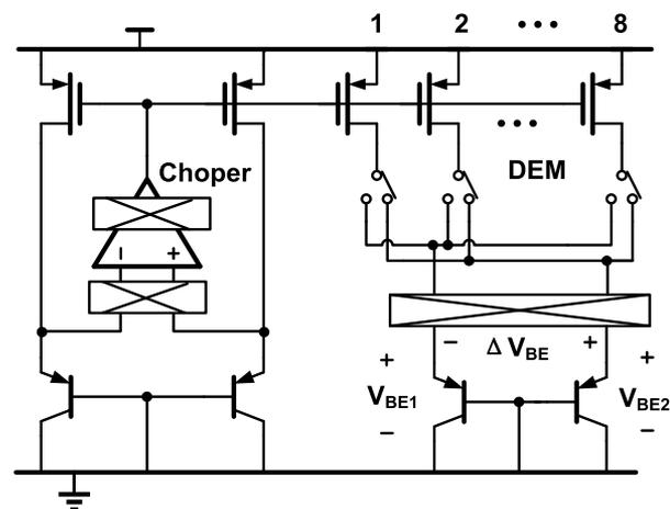
Fig. 10. Schematic diagram of the on-chip temperature sensor.
