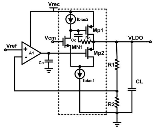
Fig. 3. Schematic diagram of the on-chip regulator.
