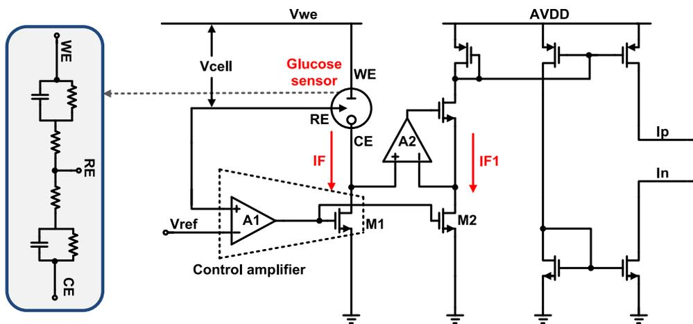
Fig. 8. Schematic diagram of the current mirror-based potentiostat.
