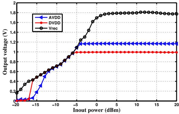
Fig. 4. Measured output voltage of rectifier and regulator versus different input power (a limiter clamps the voltage below 1.8 V).
