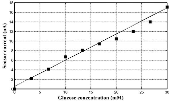
Fig. 18. Measured sensor current versus glucose concentration.
