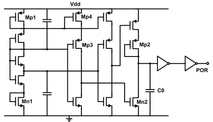
Fig. 7. Schematic diagram of the POR.
