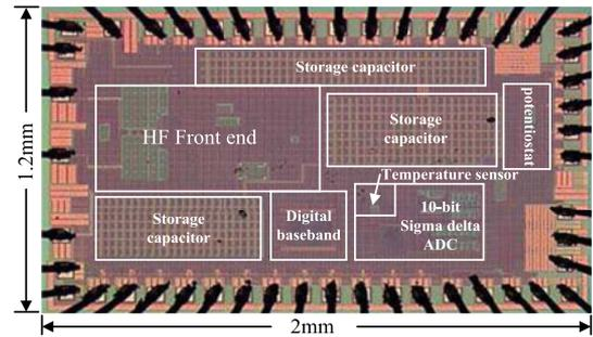
Fig. 16. Chip microphotograph of the proposed circuits.
