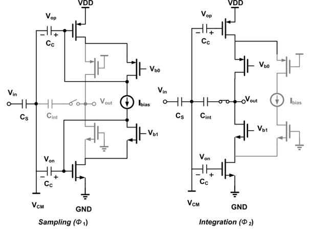
Fig. 12. Schematic diagram of the inverter-based OTA.
